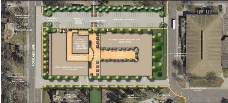
This rendering shows the front structure, along Portland, is an L-shaped four-story apartment building over a two-story garage. The U-shaped building would be a five-story apartment building over a one-level garage, and the square building, in between, is a two-story restaurant and banquet hall over a two-level garage. Motorists would access the parking garages from south-side entrances.
