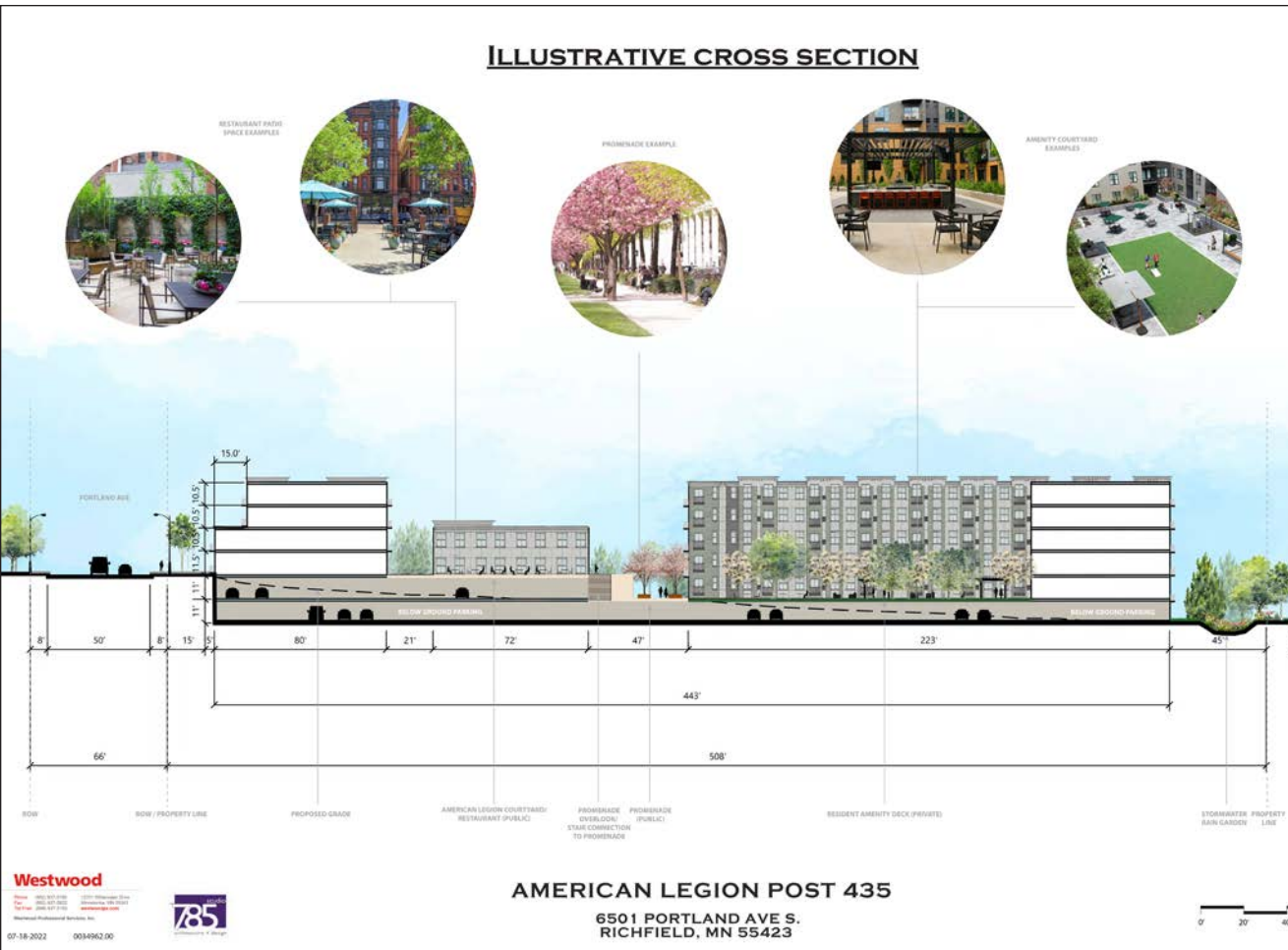
This cross-section rendering of the Post 435 site shows the parking lot beneath and how the buildings sit on the site's downhill slope.
