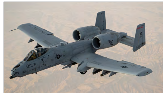
The A-10 Warthog is known for the fearsome 30 mm, seven-barrel Gatling gun mounted on its nose. Called the GAU-8/A Avenger, it fires armor-piercing depleted uranium and high explosive incendiary rounds.
